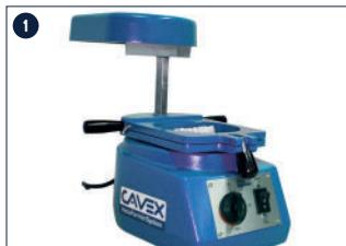
Turn the heating element to the back. Place the frame that holds the plate slightly above the part with the holes.
