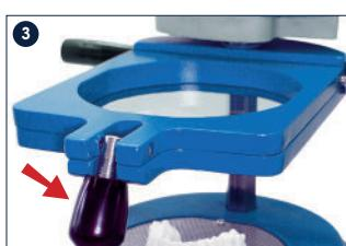
Close the frame and tighten the black knob. Then slide the frame all the way up until it touches the grey part. Turn the heating element above the frame.
