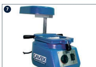
Let the device thermoform for 30 seconds, then turn off the vacuum pump and allow it to cool for about 2 minutes. Then loosen the frame and carefully remove the plate with the dental arch model.
