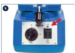
Set the push button up to the 'HEATING' position and give the timer a firm turn. The light above will turn on. Set the timer to more than 4 minutes.
