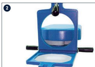
Remove the blue foil from the Bleach thermoforming plate and then place it in the frame.
