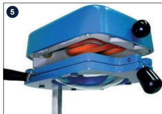
Place the dental arch model in the center of the part with the holes. The Bleach thermoforming plate will heat up and slowly sag. Make sure the dental arch model is positioned in the center on the vacuum plate with holes.
