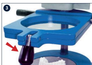
3 Close the frame and tighten the black knob. Then slide the frame all the way up until it touches the gray part. Rotate the heating element over the frame.
