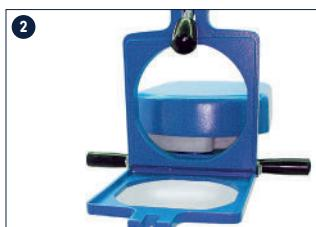
2 Place the Mouth protector thermoforming sheet in the frame with the transparent side facing up.
