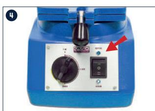
4 Set the lever to 'HEATING' and turn the timer generously. The light above will turn on. Set the timer for more than 4 minutes.
