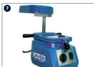
7 Let the device vacuum-form for 60 seconds, then turn it off and allow it to cool for about 2-3 minutes until it no longer feels sticky. Then loosen the frame and carefully remove the sheet with the dental arch model.
