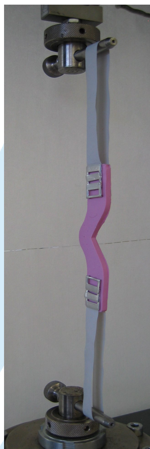
Fig 1. Sample before testing the tensile strength with Instron® 500.
